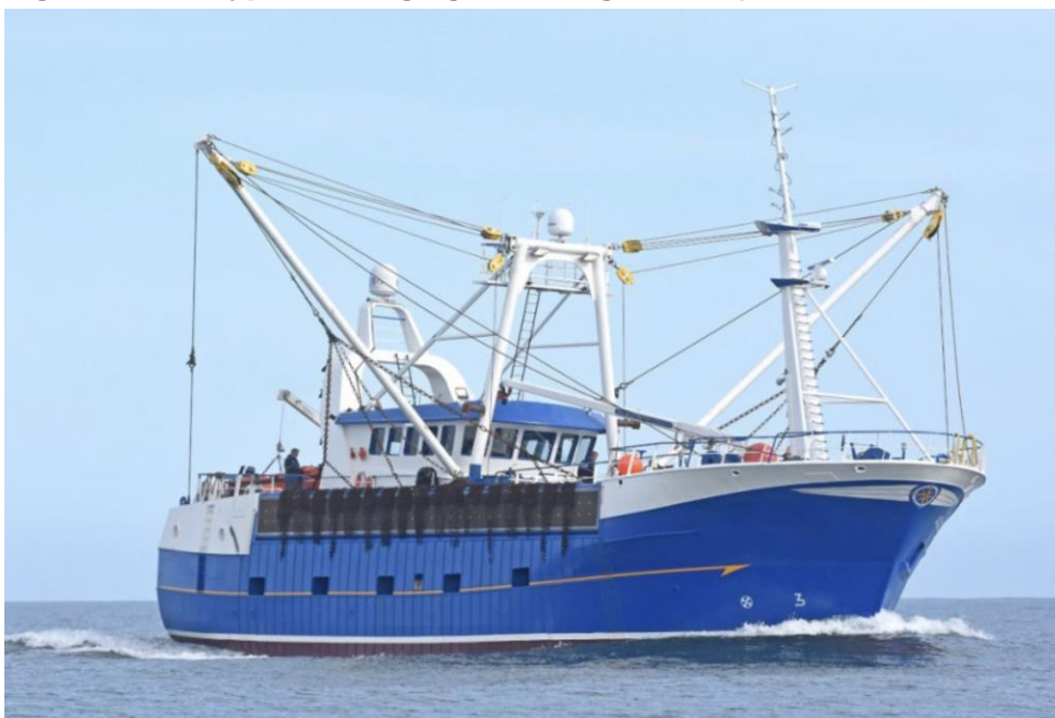
Figure 3.93.9 Example of dredge vessel (Source: Fishing News)
